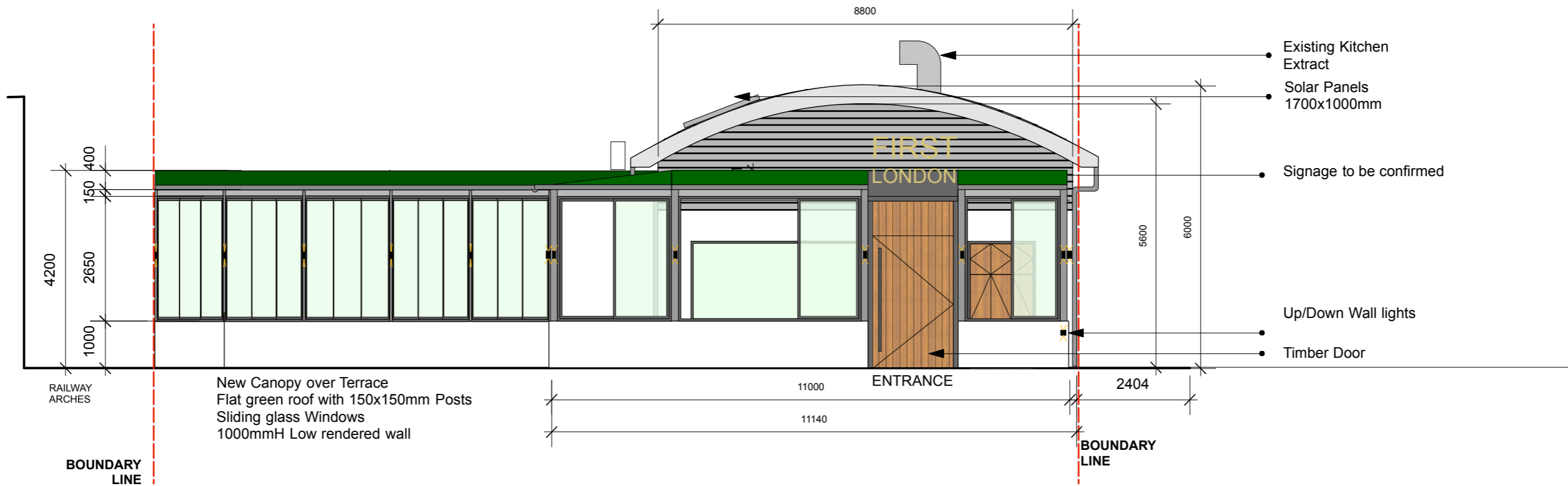
Proposed Front External Elevation ( Windows when premises is Opened )
